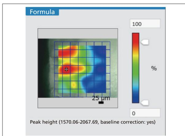
Fig. 3 Mapping Image Obtained at Corrected Peak Height of Around 1750 cm<sup>-1</sup>
