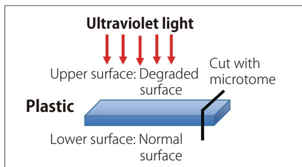
Fig. 1 Flat Cross-Sections from Degraded PP Plastic
