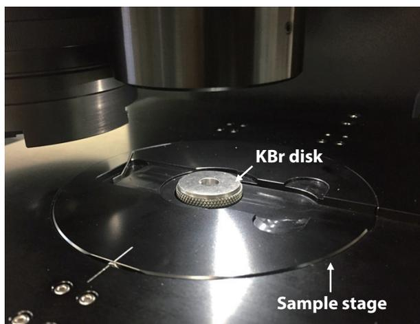
Fig. 4 KBr Disk Set for Measurement
