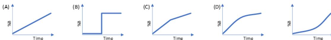
Figure 2 Schematics of different gradient profiles; (A) linear, (B) step, (C) segmented and (D) curved profiles
