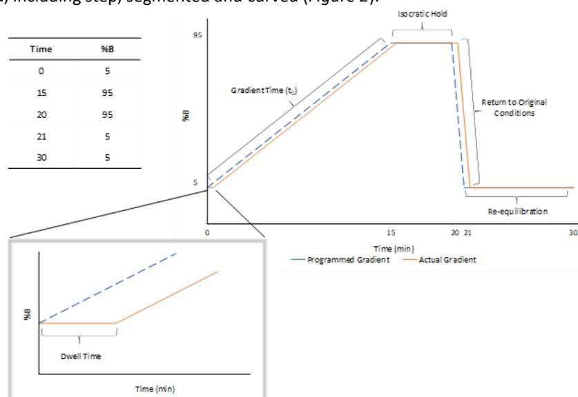
*Figure 1* Schematic of the programmed gradient, with the corresponding gradient timetable and the actual gradient
