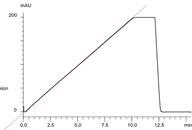
*Figure 1* Operating conditions for the pump linearity test and a corresponding chromatogram with a line to illustrate linearity throughout the entire gradient.
