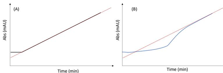
Figure 2 Schematic of (A) the linear response at the lower percentage composition and (B) the deviation of the pump linearity at the lower percentage composition.
