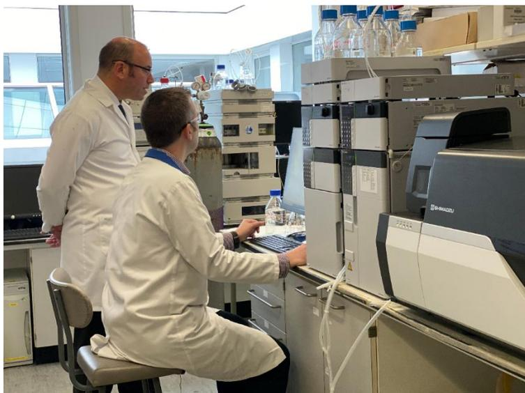
The LCMS-8060 features a triple quadrupole mass spectrometer allowing high throughput analysis which hugely benefits research labs producing large amounts of data. For example, the team at KCL run over 280 injections per day with a 5-minute run-time. "For us, the speed of the instrument means we can run rapid gradient LC separations and still maintain very high data acquisition frequencies (>20-30 datapoints per peak) for at least two
