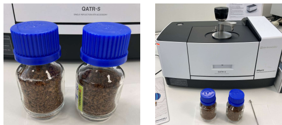
Fig. 2: classical instant coffee available with and without caffeine filled from the commercial glass into the two glass bottles at left and in back at right the view to the IRSpirit-T with diamond-based QATR-S accessory.
