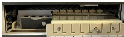
Some of the Shimadzu equipment used at Exscientia for reaction monitoring: (top) the analytical LC-MS, and (bottom) the flow-through vial configuration, which physically connects to the chemistry platform.
