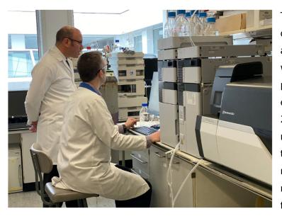
The LCMS-8060 features a triple quadruple mass spectrometer allowing high throughput analysis which hugely benefits research labs producing large amounts of data. For example, the team at KCL run over 280 injections per day with a 5minute run-time. "For us, the speed of the instrument means we can run rapid gradient LC separations and still maintain very high data acquisition frequencies (>20-30 datapoints per
