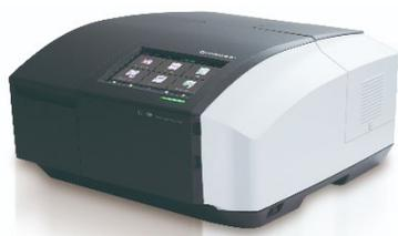
Fig. 1 UV-1900i UV-Vis Spectrophotometer
