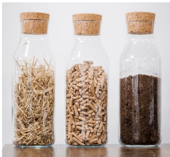
Straw, wood pellets and compost – just three of the biomass feedstocks that the team at Wild Hydrogen have been investigating for hydrogen generation.
