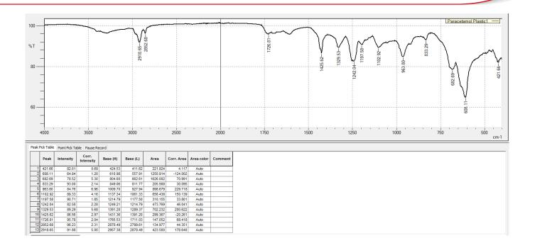
Now the peaks are labelled the correlate the wavenumber to a characteristic group table to identify the likely plastic component in the pharmaceutical packaging.
