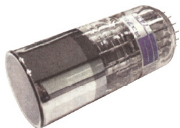
Fig. 9 End-On Photomultiplier Tube
