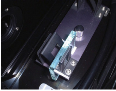
Fig. 2 5 mm Thick Glass Plate Placed in Standard Sample Compartment (film holder)
